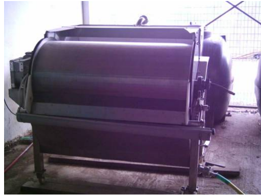
Rotating screen (250 µm)
