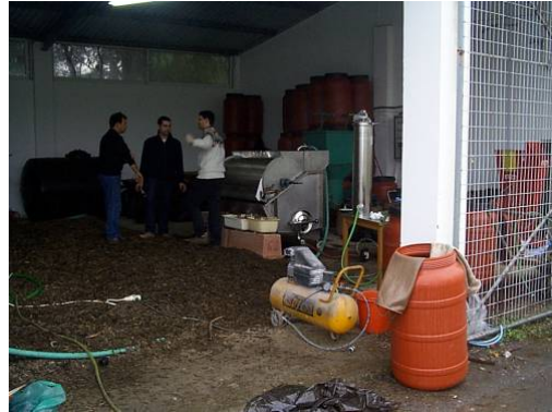
Wastewater filtering Trials (rotating screen and bagfilter)
