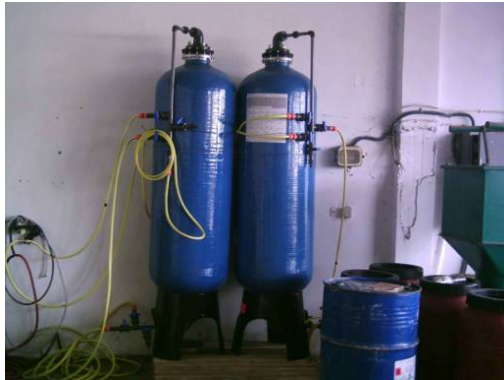
Polyphenols extraction using selective adsorbance resins
