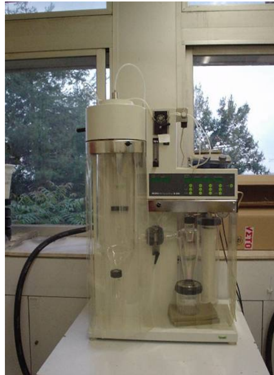
Final formulation of the polyphenols extract in a spray drier
