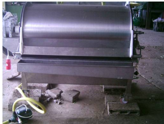
Rotating screen (100µm)
