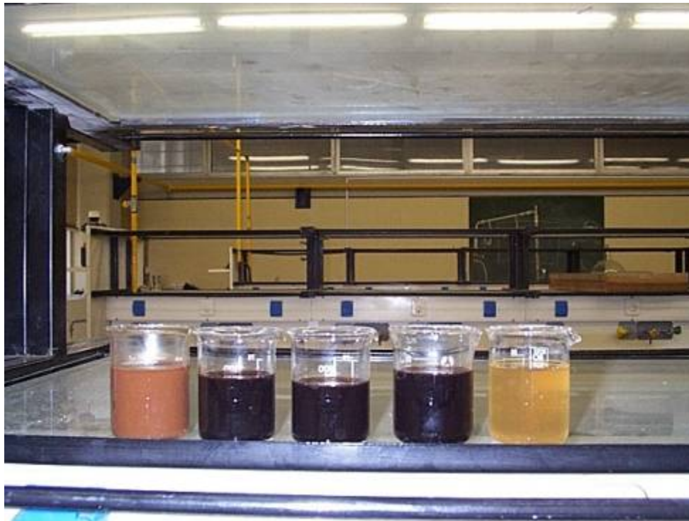
Olive oil mill wastewater evolution through the successive pilot plant process steps (from left to right-final outflow)
