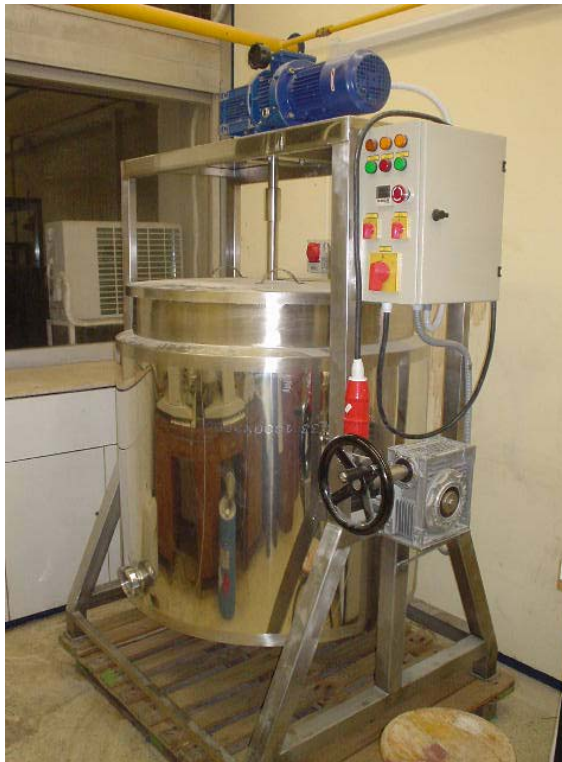
Processing of waste olive leaves in a solid-liquid extraction vessel
