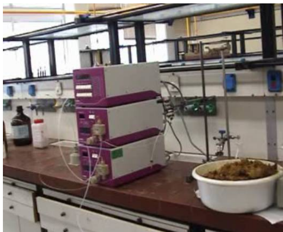
Final polyphenols purification using chromatographic techniques
