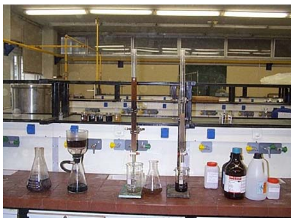
Wastewater filtration, Polyphenols capture by using resins, Regeneration of the resins using organic solvents
